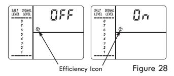
**SALT EFFICIENCY:** When this feature is ON, the water softener will operate at salt efficiencies of 4000 grains of hardness per pound of salt or higher. The softener may recharge more often using smaller salt dosage and less water. This softener is shipped with the efficiency feature set OFF. Installations in the State of California require this setting to be turned ON. Use the  $\triangle$  UP or  $\nabla$  DOWN buttons to change between OFF and ON.
