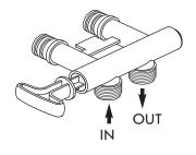
If connecting to floor level plumbing, install the bypass valve turned downward, as shown.
