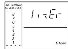
■ **Gallon or Liter readings:** Water usage and flow displays are shown in gallons. If you prefer to have the same displays in liters, press the UP button until Liter shows.
