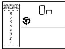
■ **SALT EFFICIENCY:** When this feature is ON, the unit will operate at salt efficiencies of 4000 grains of hardness per pound of salt or higher.
