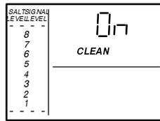
■ **CLEAN:** This feature is beneficial on water supplies containing iron and/or high amounts of sediments (sand, silt, dirt, etc.). When set to ON, a backwash and fast rinse cycle will occur first, preceding the normal regeneration sequence (see page 2-4). This provides extra cleaning of the resin bed before it is regenerated with the salt brine. To conserve water set this feature OFF if your water supply does not contain iron or sediments.
