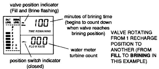
**POSITION SWITCH STATUS:** With the valve in service, or any of the recharge cycles, the switch indicator will show open  $\rightarrow \swarrow$ . While the valve is rotating from 1 position to another, the indicator will show the switch closed  $\rightarrow \searrow$ . A defect is probable if indications vary from this pattern.
