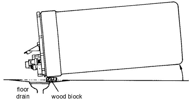
7. Looking at FIG. 12, lay a piece of 2 inch thick board near the floor drain. Move the softener close to the drain. SLOWLY and CAREFULLY, tip it over until the rim rests on the wood block with the inlet and outlet over the drain. **Do not allow the softener's weight to rest on the inlet and outlet fittings or they will break.**
