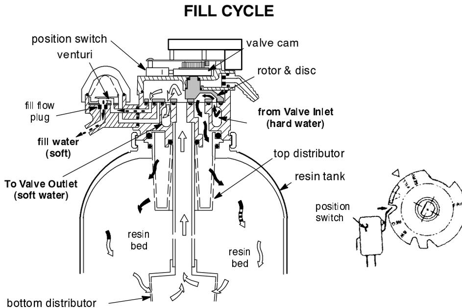
To begin a regeneration, the electronic timer energizes the circuit to the valve motor. The valve motor rotates the rotor and disc and the valve cam until the position switch lever drops, to open the motor circuit and position the valve in FILL. As the rotor and disc rotates, the port opens for SOFT water fill through the venturi. Fill flow continues to the brine valve, and into the salt storage tank. Soft water is still available to the house lines.
