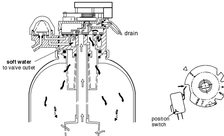
During FAST RINSE, the rotor & disc is positioned so water flow enters the resin tank through the top distributor, and exits through the bottom distributor, to the drain.
