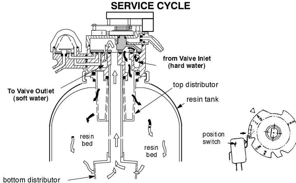
Hard water enters the valve inlet port. Internal valve porting routes the water down and out the top distributor, into the resin tank. Hard water is softened as it passes through the resin bed, then enters the bottom distributor. Soft water flows back into the valve and out the valve outlet, to the house soft water pipes.
