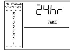
■ **12 or 24 hour clock:** All time displays are shown in standard clock time (1 to 12 PM; and 1 to 12 AM) at the 12 hr default setting. If military time displays are desired, set to 24 hr by pressing the UP button.
