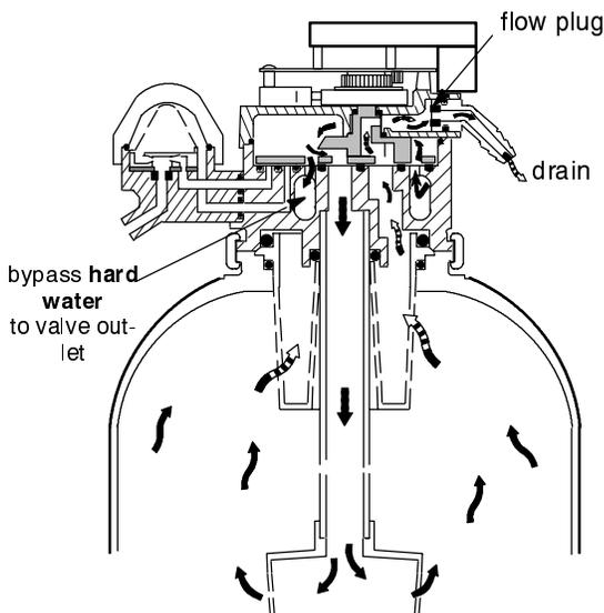
Timer/switch action again allows the motor to turn the rotor & disc to place the valve in BACKWASH, stopping water flow to the nozzle. Water is routed down and out the bottom distributor, up through the bed, and out the top distributor to the drain. The fast flow (controlled by a flow plug in the drain fitting) flushes dirt, sediments, iron deposits, remaining brine and hardness to the drain.
