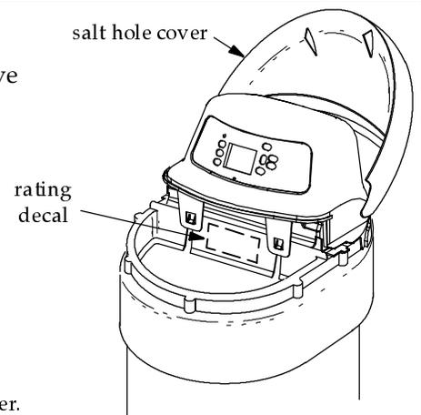
† The model number is on the rating decal, located on the rim, under the salt hole cover.
