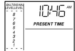
Each press of the UP /DOWN buttons changes the time by 1 minute. Holding the buttons in changes the time rapidly.
