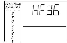
This code identifies the softener nominal capacity size. If the wrong number shows, the softener will operate on incorrect programming. Do the following as needed.
