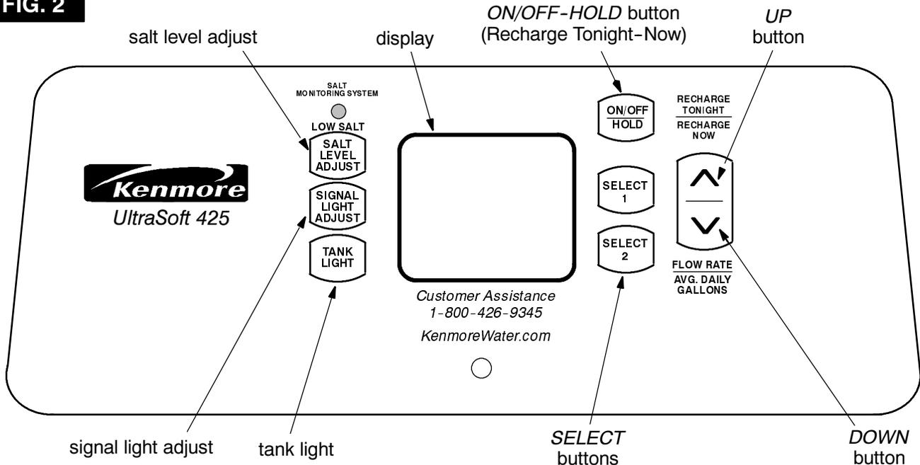
When the transformer is plugged in, the model code HF36, and a test number (example: A2.4) show in the face plate display for 4 seconds. Then, 12:00 AM and *PRESENT TIME* begin to flash.
