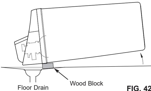
7. Move the softener close to the drain. Slowly and gently, tip it over until the rim rests on the wood block with the inlet and outlet over the drain. Do not allow the softener's weight to rest on the inlet and outlet fittings or they may break.
