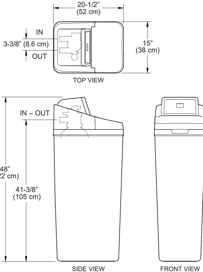
**NOTE:** Due to variances in production and assembly, the water softener valve height may vary by up to 1/2", and may not match previously installed systems. This will not affect system performance.
